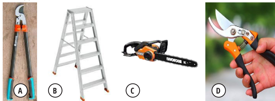
Figure 3.1 Some equipment that are used in the citrus pruning process: lopper (A); ladder (B); small chainsaw (C); secateur (D).
